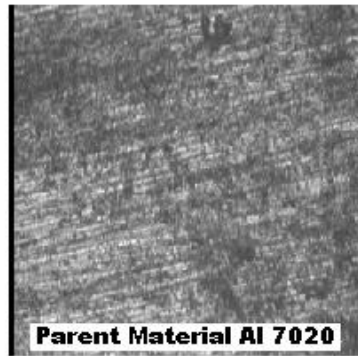
Fig. 2 Micro image of Al 7020.
