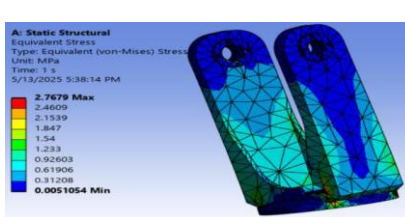
Fig. 10: Max stress at 80
